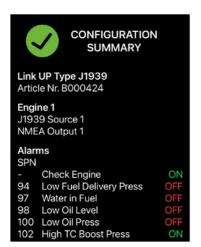
2. After the readout, the App will show the "Configuration Summary", which displays all the current settings of the device.
