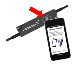
1. Launch the "Link Up Configurator" App and read the actual configuration of the LinkUp device by "tapping" the smartphone onto the LinkUp wireless area (indicated by the red arrow).
